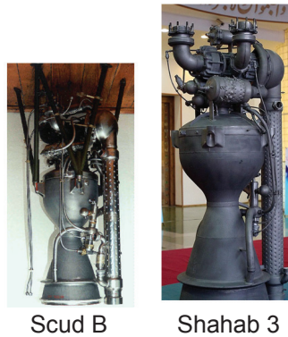
Figure 5.6 Scud B and Shahab 3 Engines (roughly in scale)
