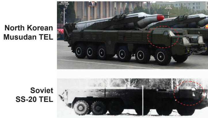
Figure 5.15 North Korean and Soviet Six-Axle TELs
