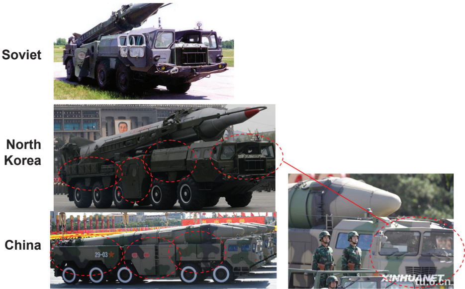
Figure 5.9 North Korean and Chinese Five-Axle TELs, Soviet Four-Axle TEL
