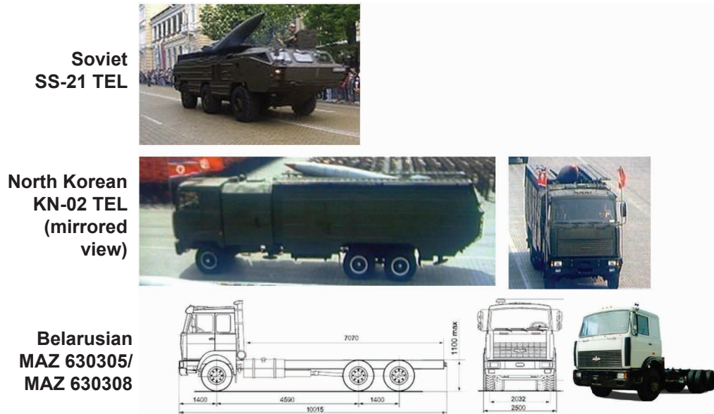
Figure 5.12 North Korean and Soviet Three-Axle TELs
